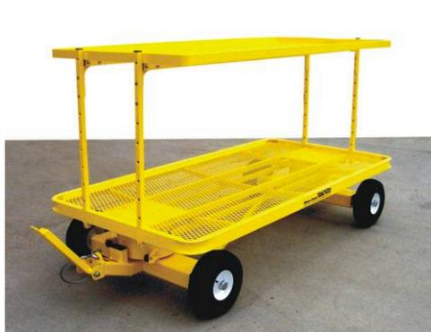
Shelves are available in a variety of sizes with either expanded metal or solid bottoms.
